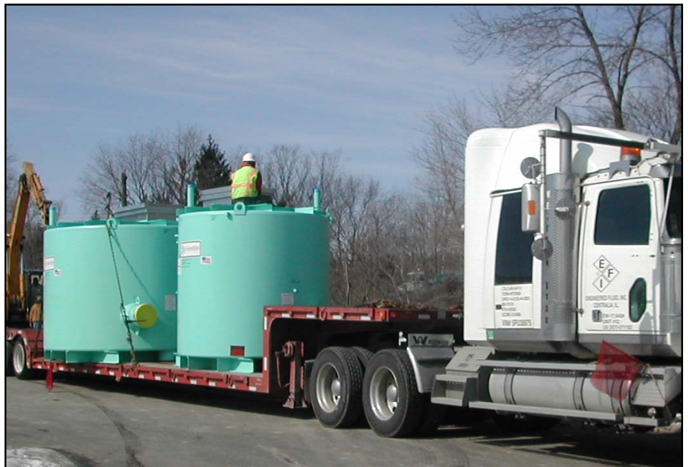
Mundelein, Illinois - two pressure reducing stations arriving at the job site on a EFI tractor trailer.
